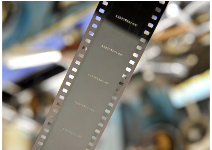
銅版字幕機的製成品 The final product made by the copper-plate printing machine
