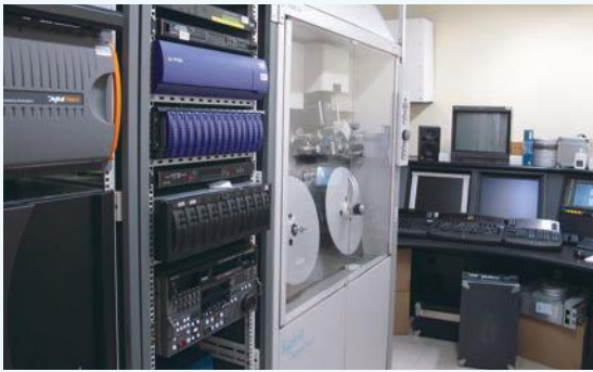
Spirit DataCine 包括主機、掃描器與 Da Vinci 控制台 Spirit DataCine including the main console, the scanner and the Da Vinci Panel
