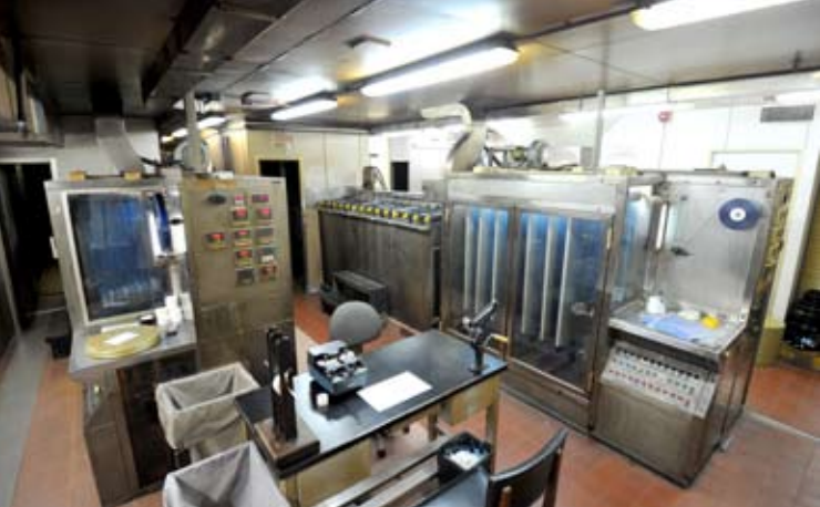
趙耀俊巧製「香港製造」的沖片機 The 'Made in Hong Kong' film processors put together by Eugene Chao.
